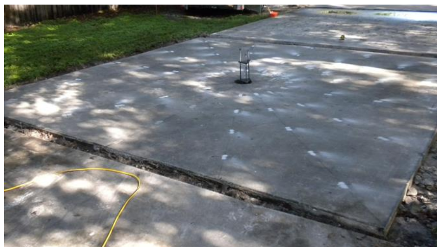
Fig. 4. Interior slab bracket test specimen
