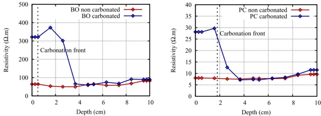
Fig. 3: Comparison between non carbonated and carbonated materials.
