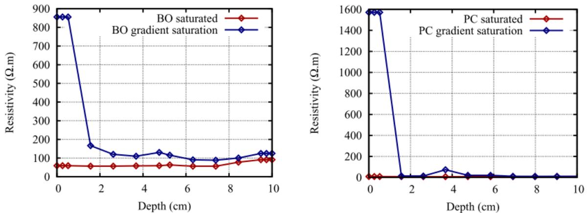
Fig. 2: Comparison between the electrical resistivity of saturated and dried materials.
