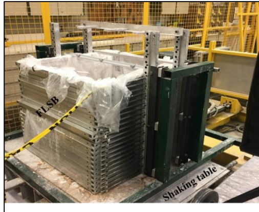
Fig. 2: Photo of the shaking table and flexible laminar shear box (FLSB) used in this research.
