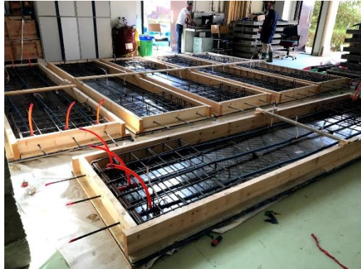
Figure 3. The six post-tensioned slab specimens before concrete casting (left) and after concrete casting (right).
