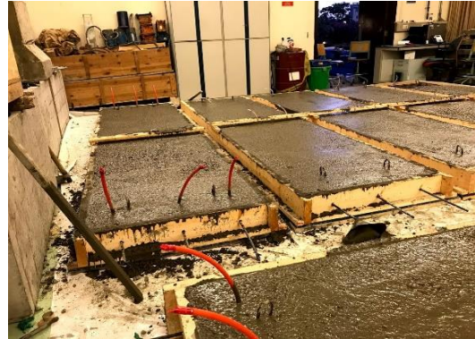
Figure 3. The six post-tensioned slab specimens before concrete casting (left) and after concrete casting (right).
