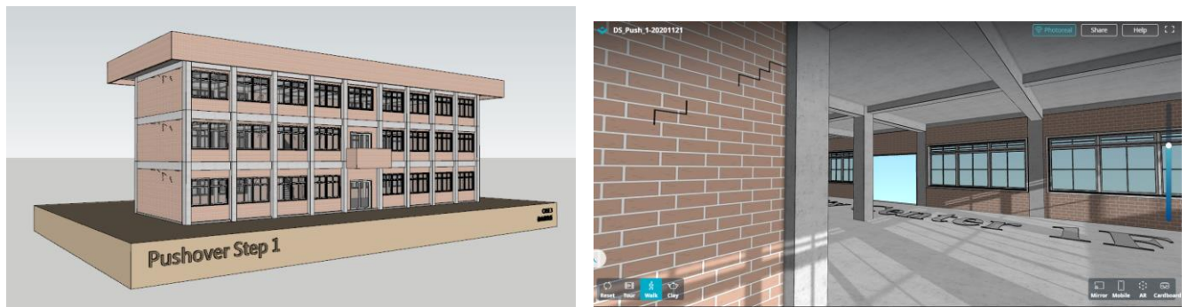
Fig. 17 Brick filled RC city hall damage simulation SketchUp and internal VR model
