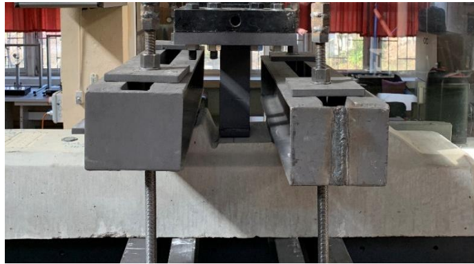
Fig. 7: Pull-out resistance test setup.
