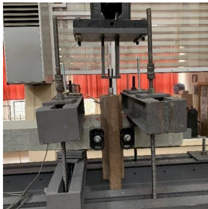
Fig. 4: Longitudinal rail restraint test setup.
