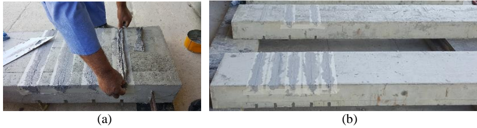
Figure 4: (a) Installing the FRP strips in the NSM grooves; (b) Strengthened Specimens.
