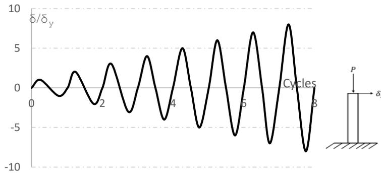
Fig. 3: Cyclic loading path protocol.
