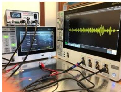
Figure 2 Experimental setup including function generator, oscilloscope, amplifier and aluminium plate
