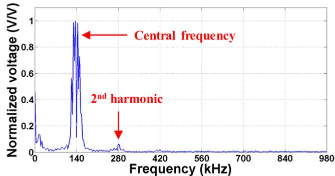
Figure 3 Experimental data captured at transducer 2 in frequency domain
