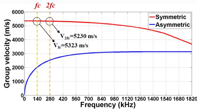
Figure 5 Group velocity dispersion curve for the plate specimen calculated by DISPERSSE
