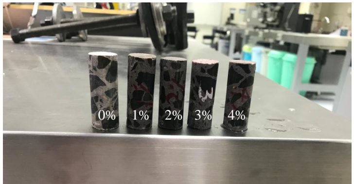
Fig. 4: Extracted cylindrical core samples – from left to right 0%, 1%, 2%, 3% and 4%
