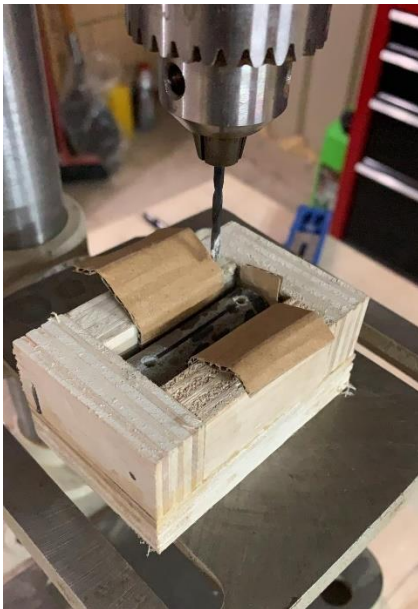
Fig. 3: Sample preparation for thermal conductivity test
