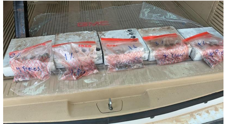
Fig. 2: 50 mm-thick slabs after waterjet cutting
