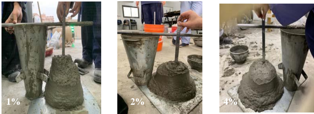
Fig. 2: Slump test for 1%, 2% and 4% PTFC
