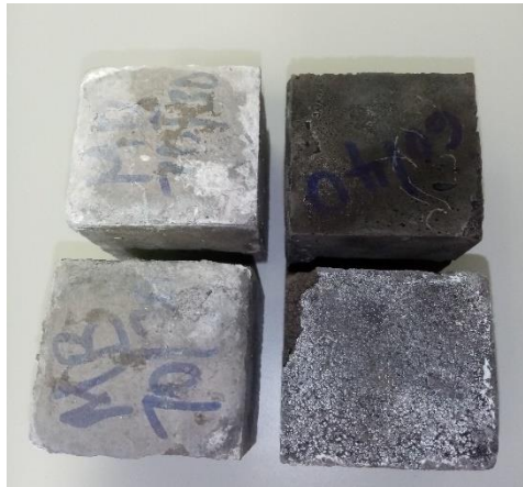
Figure 4: Cube sample efflorescence
