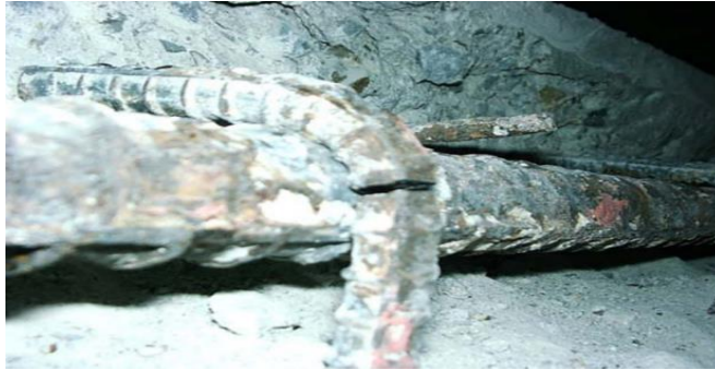
Fig. 1: Example of fractured steel bar.
