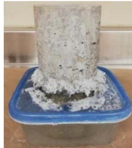
**Figure 2.** Salt efflorescence in the dry portion during exposure.
