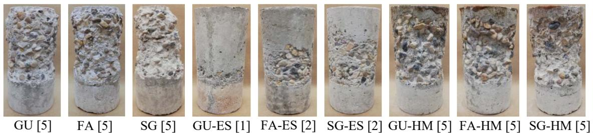
**Figure 1.** Uncoated and coated specimens at the end of PSA exposure.
