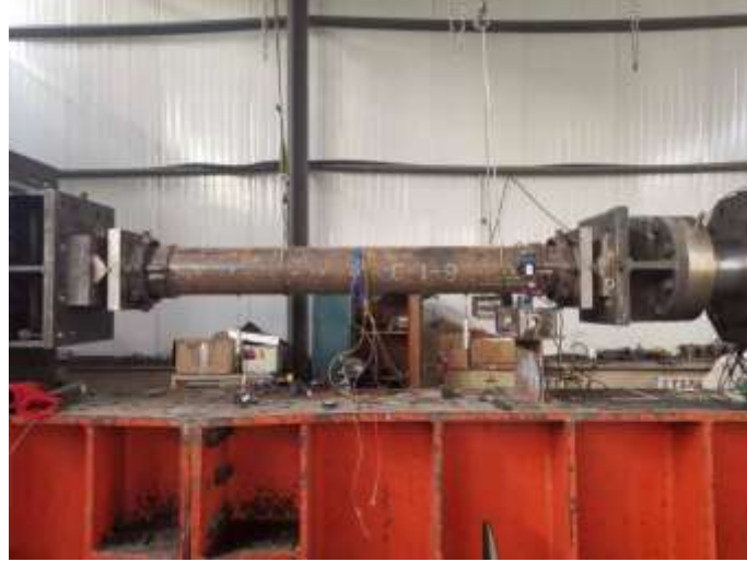
Fig. 2: Test setup of CFDST slender column under axial compression.
