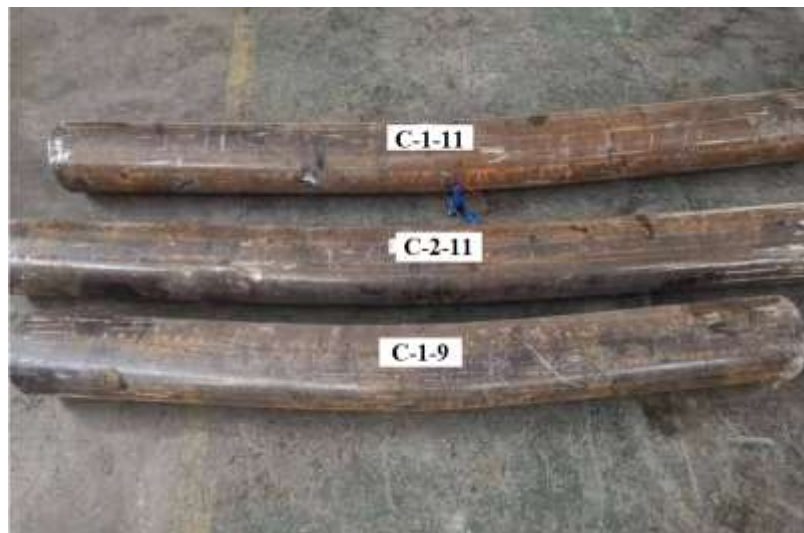
Fig. 3: Typical failure mode of circular CFDST slender columns under axial loading.
