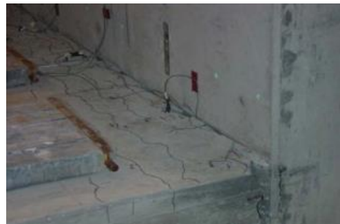
Fig. 2: Post-tensioned slab cracking at 5% drift
