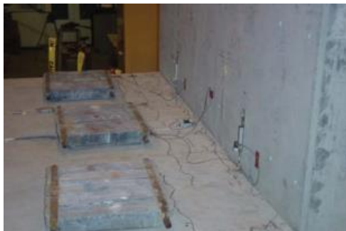
Fig. 1: Post-tensioned slab cracking at 0.5% drift
