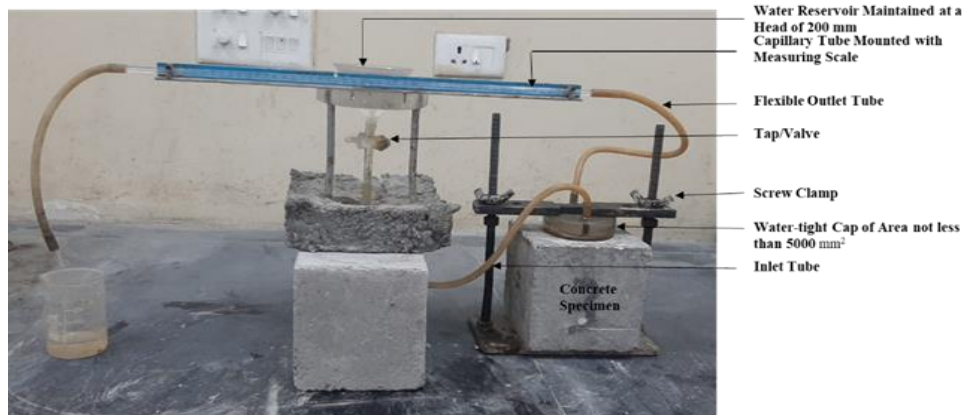
a) Capillary Suction Test Setup
