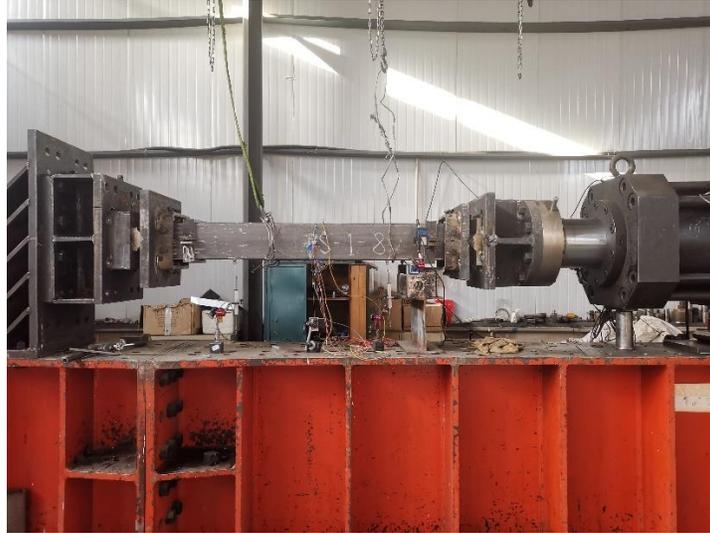
Fig. 2: Typical test setup of square CFDST slender column under concentric loading.
