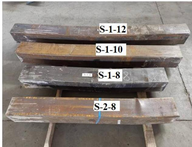
Fig. 3: Typical failure mode of square CFDST slender columns under concentric loading.
