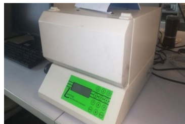
Fig 3: Laser Comp heat flow meter instrument (Fox200).
