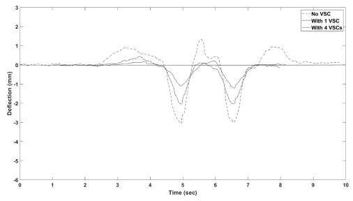
Fig. 6: Vertical deflection of sleeper, obtained by VB system, before VSC, after installation of 1 VSC, and after installation of 4 VSCs.
