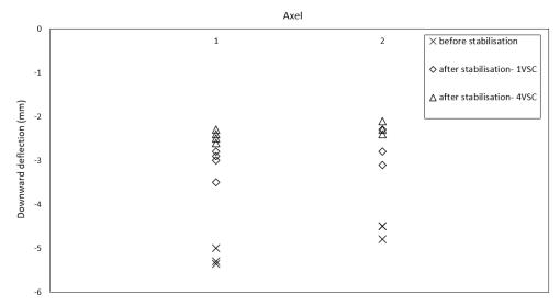
Fig. 4: Maximum downward deflection of the rail at fishplate under repeated vehicle passage load with 34 tones based on various vehicle passage, before and after stabilisation.
