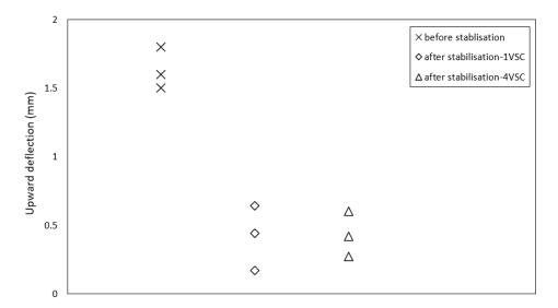
Fig. 5: Maximum upward deflection of the rail at fishplate on repeated vehicle passage, before and after stabilisation.
