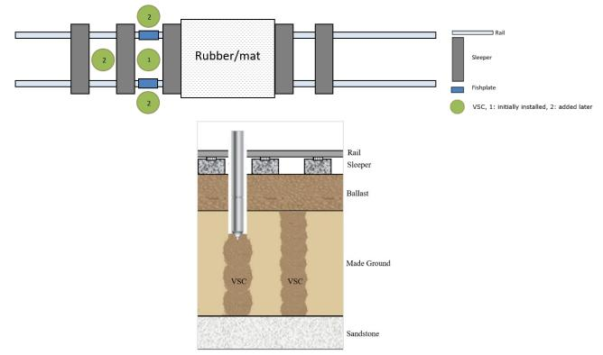
Fig. 1: Schematic of dry vibro-replacement method for stabilizing trackbeds with stone columns; plan view (top) and section view (bottom).
