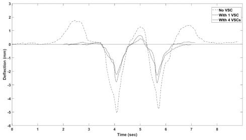
Fig. 3: Vertical deflection of rail at fishplate, obtained by VB system, before VSC, after installation of 1 VSC, and after installation of 4 VSCs.
