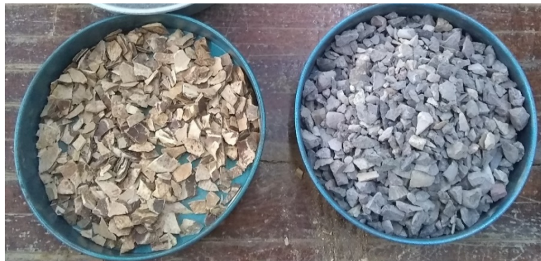
Fig. 1: Appearance and comparison of CS and crushed aggregate particles.
