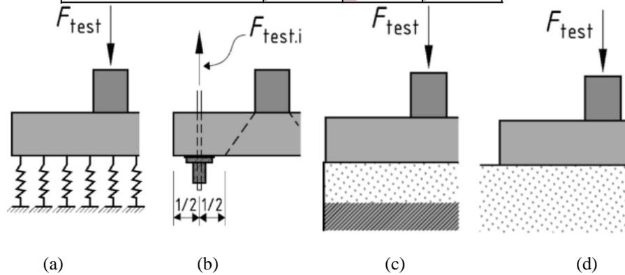
Figure (2) Subsoil model types: a) springs; b) line support; c) on-soil and d) sand box
