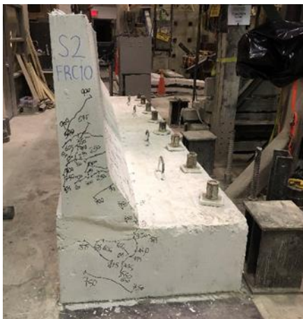
Fig. 10: Crack pattern at end of specimen S2-FRC10
