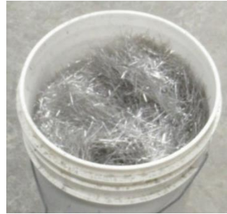
(b) Fibers before adding them to concrete mix
