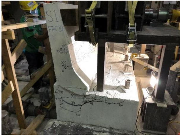
Fig. 8: Concrete breakout failure in the deck (S1-FRC10)
