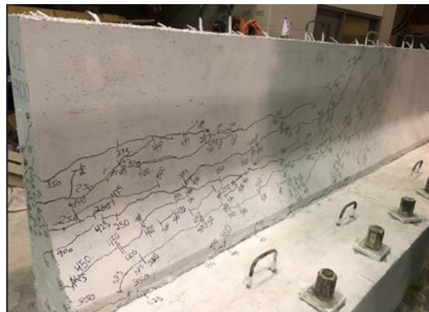
Fig. 11: Trapezoidal tension-flexural shear crack pattern (S2-FRC10)
