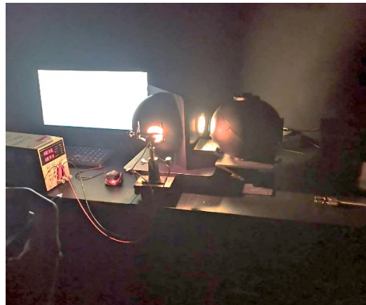
Figure 4: Apparatus for light transmission test
