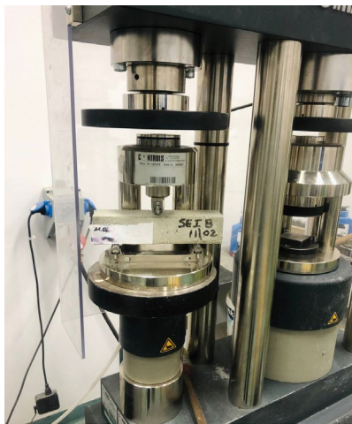
Figure 2: Flexural strength test
