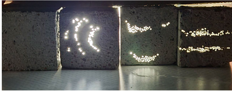
Figure 3: Samples ready for light transmission test
