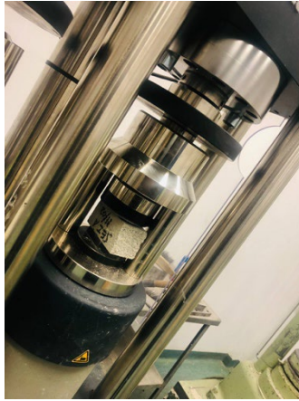
Figure 1: Compressive strength test
