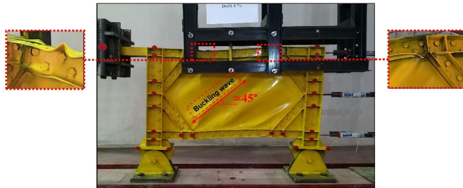
Fig. 6: The test specimen's deformation and failure at 4% drift.
