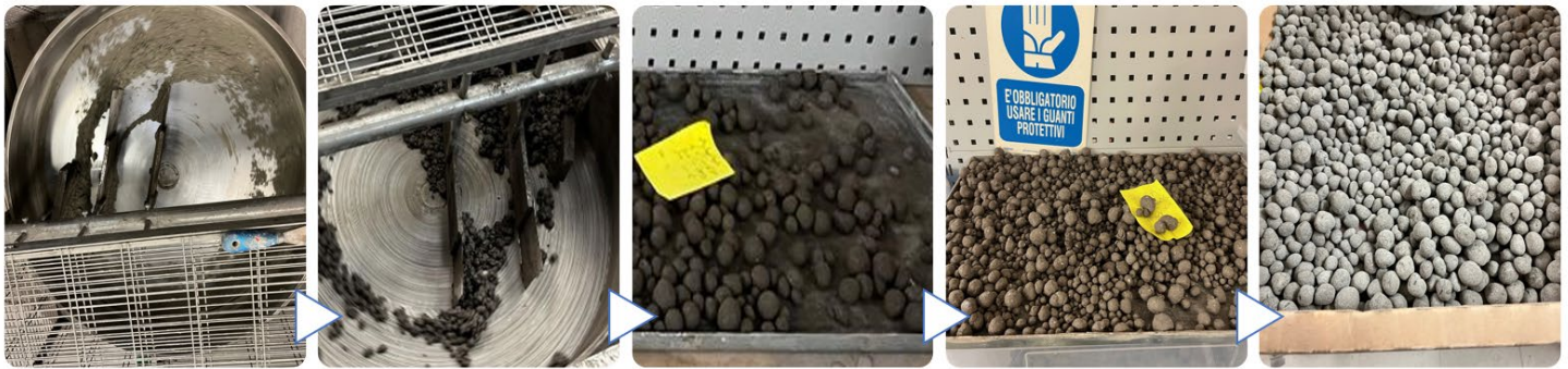
Figure 3 Process of obtaining granules by palletization process
