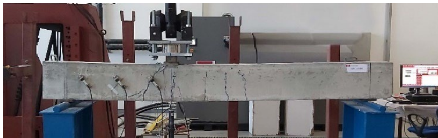
Fig. 5: A physical beam during testing
