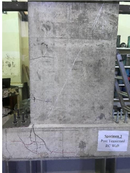
Figure 5: Failure mechanism of PTW
