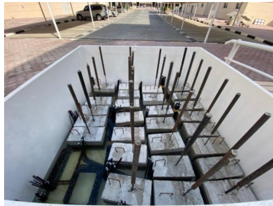
Fig. 2: Test Setup for a) bent GFRP test; b) Outdoor Marine.
