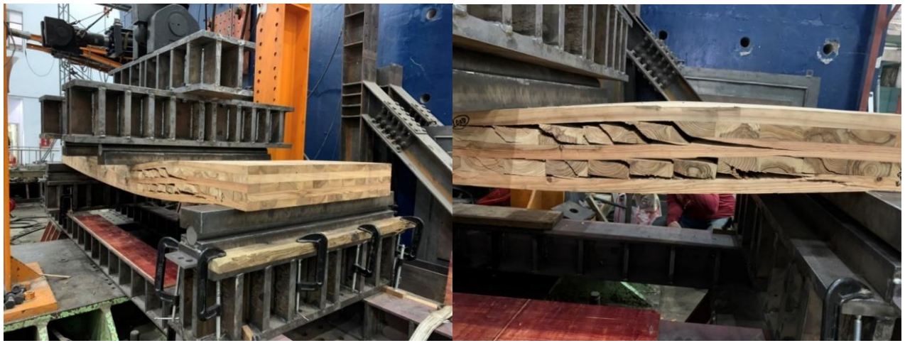
Fig. 7: Typical failure mode of CLT-2: failure form rolling shear
