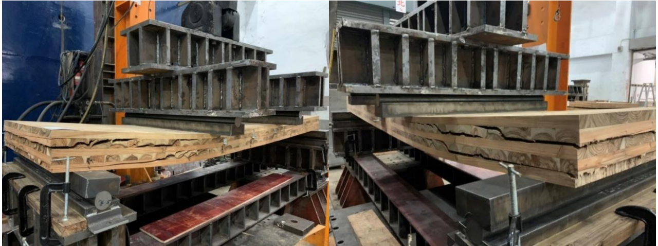
Fig. 6: Typical failure mode of CLT-1: combined failure form rolling shear and glued layer
