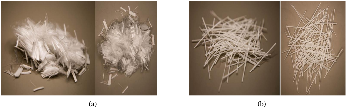
Fig. 3: Fibres uses in the study include a) Polypropylene micro fibres, b) Polyolefin macrofibres
