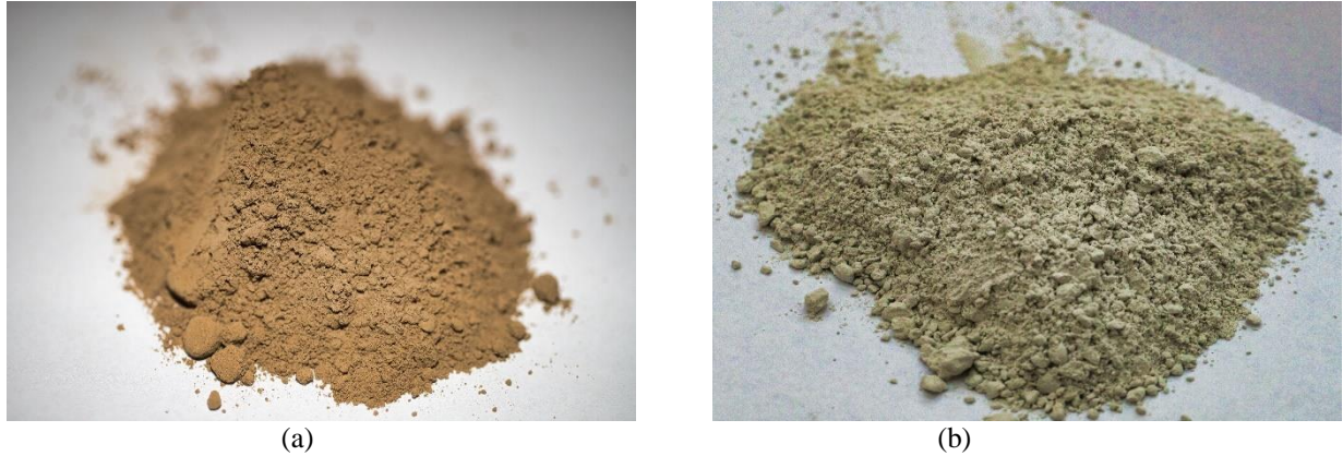
Fig. 1: Binders used in the study including (a) fly ash, (b) ground granulated blast furnace slag.
