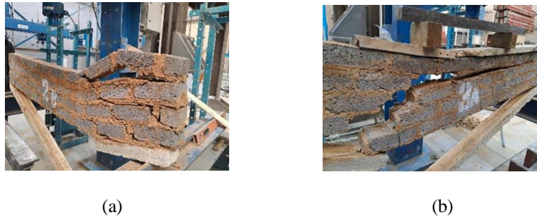
Fig. 4: Typical crack propagation arrangements along the masonry wall Lintel
