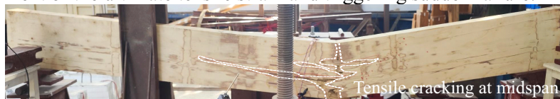
Fig. 3: Failure mode of specimen S-0.
