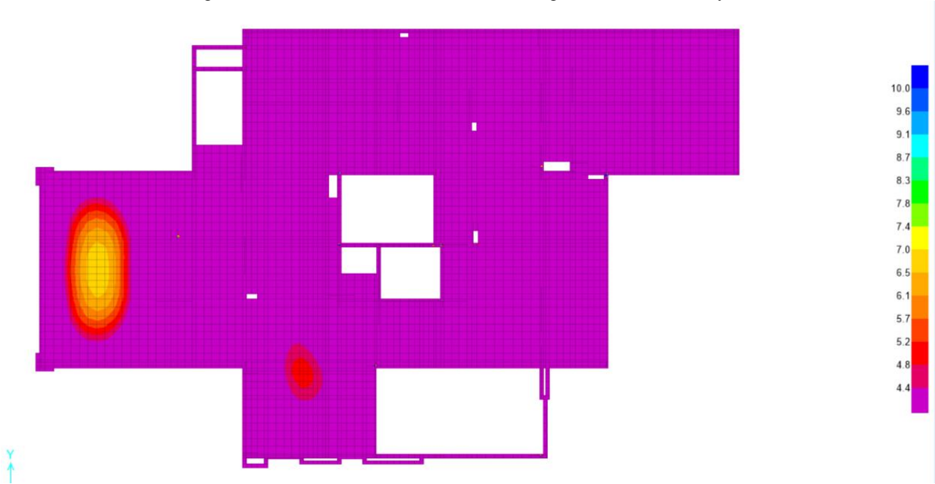
Fig 4:Bottom reinforcement in Y-direction using Finite Element Analysis
