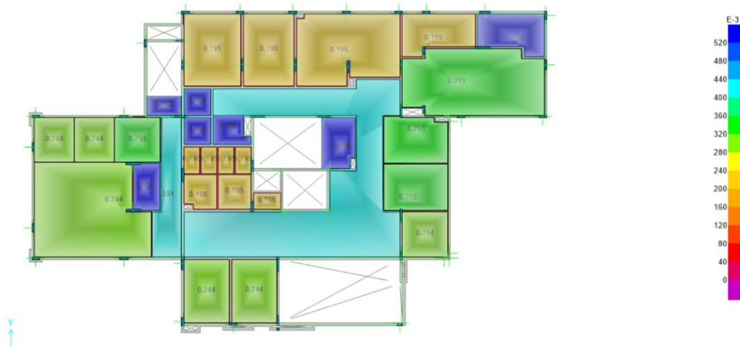
Fig 3: Animal hospital first slab plan showing live load distribution (Case 2)
