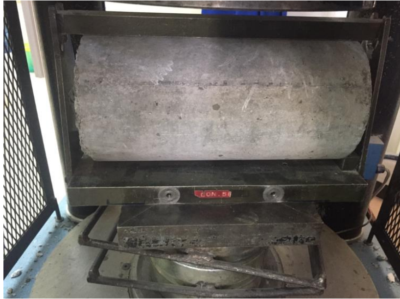
Fig. 3.1: Splitting tensile strength testing set up
