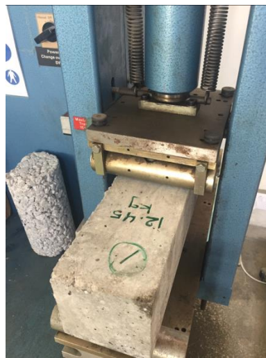
Figure 3.2. Flexural strength test set up
