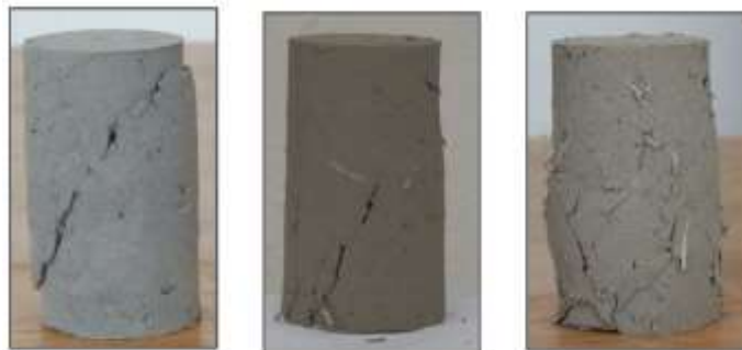
Fig. 3. Disturbed samples after UCS test (0%, 1% and 2% of fibres).
