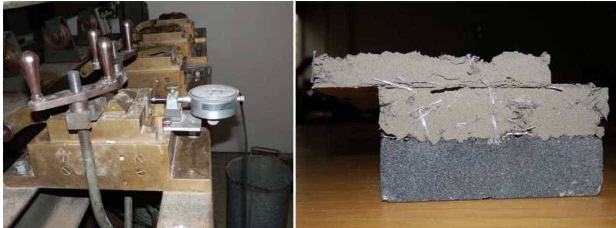
Fig. 4. Testing apparatus (left) and reinforced sample after the test (right).
