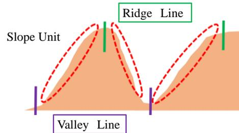
Fig. 4: Image of slope unit
