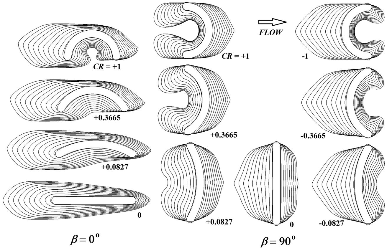
Figure 4: Effect of  $CR$  on curved plates with  $\beta = 0^\circ$  and  $\beta = 90^\circ$ .
