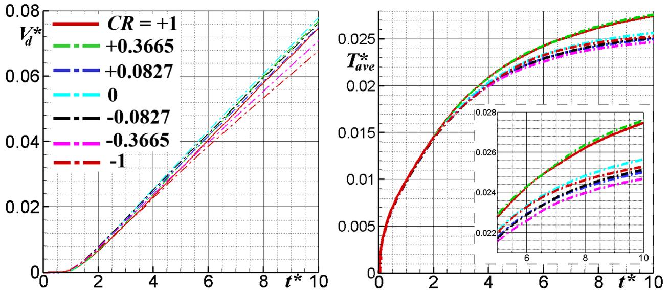
Figure 3:  $V_d^*$  and  $T_{ave}^*$  for curved plates with  $\beta = 0^\circ$ .
