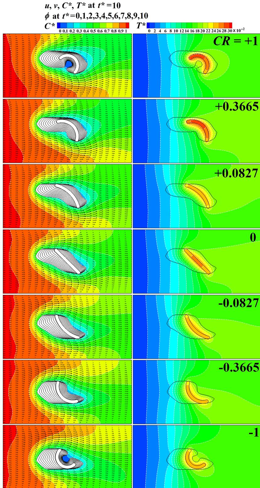
Figure 2: Effect of  $CR$  on deposition on curved plates with  $\beta = 0^\circ$ .
