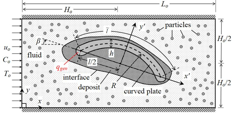
Figure 1: Schematic of a curve plate in a channel.
