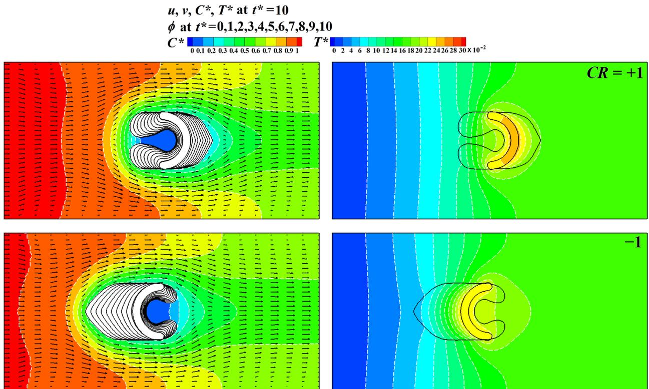
Figure 7: Effect of  $CR$  on deposition on curved plates with  $\beta = 90^\circ$ .
