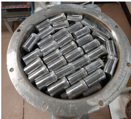
Fig. 2: (a) Schematic of flow through the experimental setup (b) in-house developed setup (c) Front-view of packed bed (d) Cylindrical capsule
