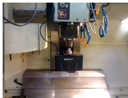
Fig.4. The Scantech scanner in the spindle of the Kondia machine.
