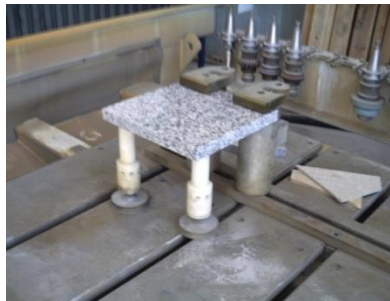
Fig.3. The fixing of granite number 1 on the stone milling center.
