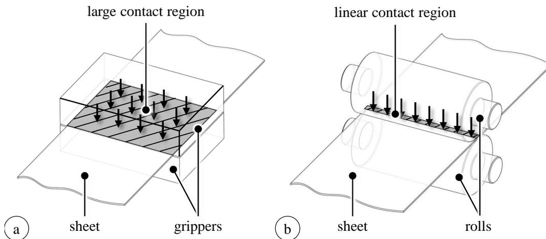
Fig. 1. Contact region in mechanical feeding systems: a) gripper feeder, b) roll feeder.
