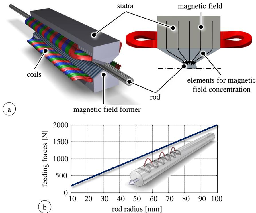
Fig. 7. Structure of a contactless feeder for rods or tubes (a) and simulated feeding forces in ferromagnetic steel depending on its radius (b).
