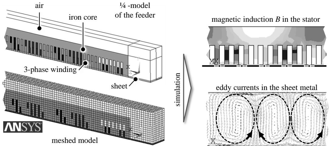
Fig. 3. FE modelling and simulation of the contactless feeder.
