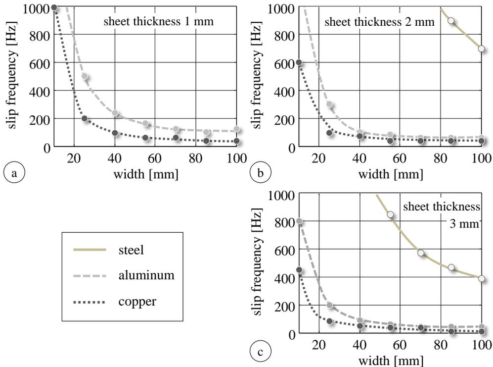
Fig. 5. Simulated optimal slip frequencies for steel, aluminum and copper in dependence on the sheet width and thickness.
