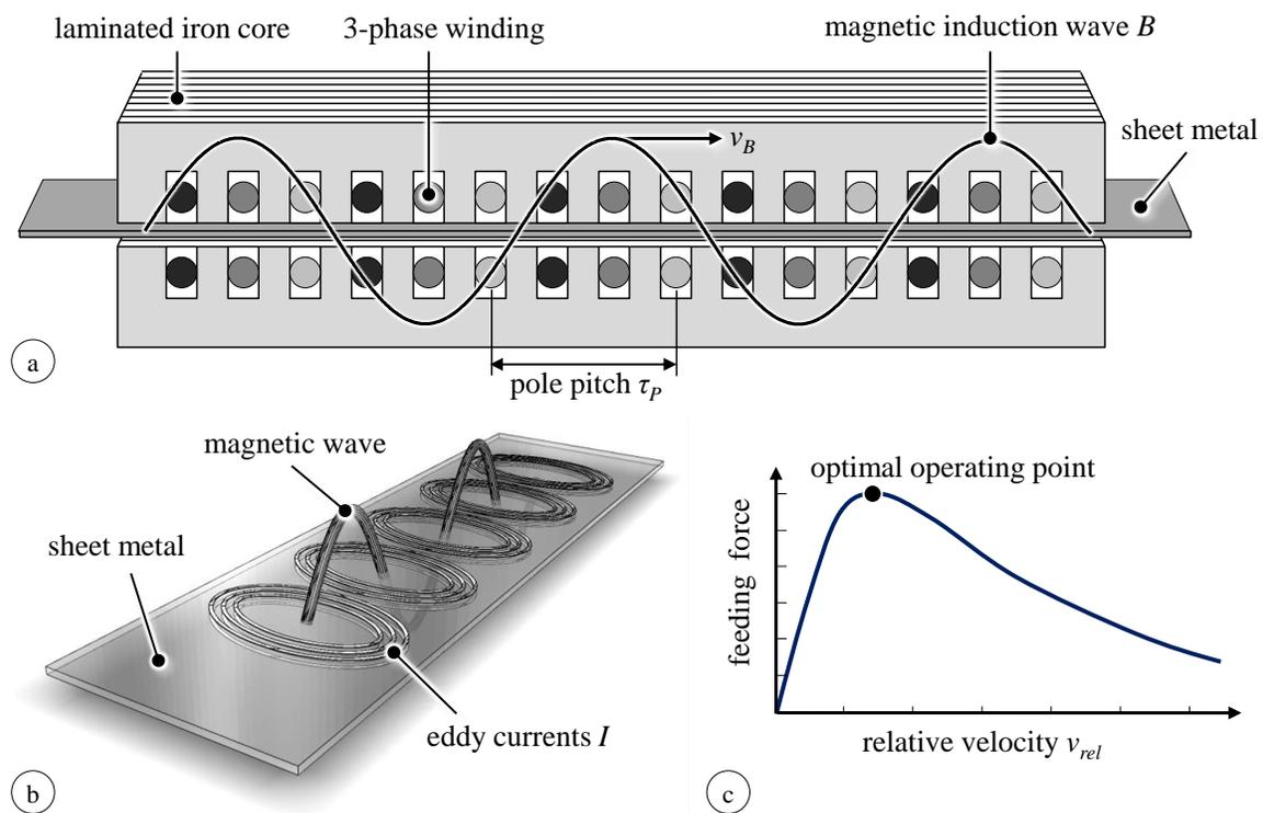
Fig. 2. Feeders structure and operational principle.
