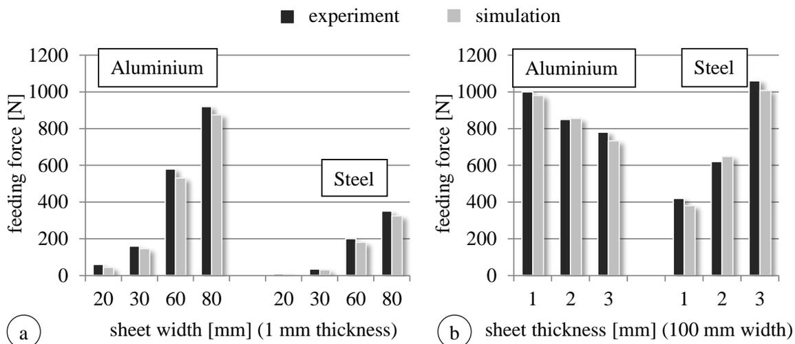
Fig. 6. Feeding forces for ferromagnetic steel and aluminum depending on the sheet width (a) and thickness (b).
