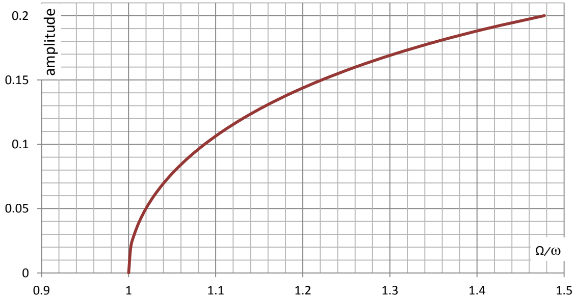
Fig. 1. Dependence of the non-linear natural frequency and the amplitude of the vibration sample chart
