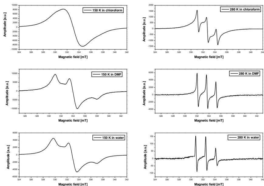
Fig. 1. EPR spectra of investigated nanoparticles diluted in different solvents and recorded at 150K and 280K temperature.
