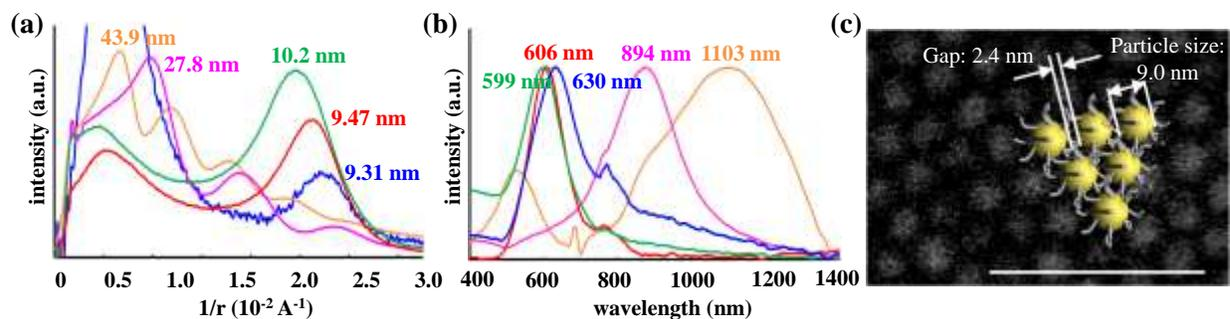
Fig. 2. (a) SAXS patterns and (b) UV-Vis-NIR extinction spectra of the 10Hex (blue), 10Dod (red), 10Hexd (green), 30Dod (magenta), and 50Dod (orange) 2D-arrays. (c) Representative illustration of the 10Dod 2D-array showing interparticle gap distance and particle size. The scale bar is 50.0 nm.
