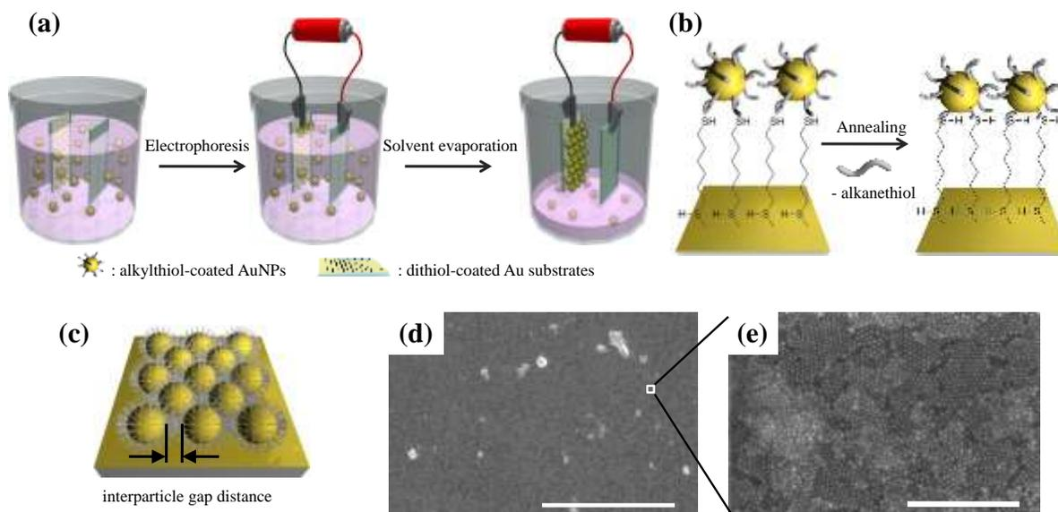
Fig. 1. Schematic illustration of (a) process of fabricating AuNP 2D-arrays, and (b) annealing process to immobilize AuNPs covalently onto substrates. (c) 10Dod 2D-array. (d) SEM images of 10Dod 2D array fabricated on 1,6-hexanedithiol-coated gold substrates by the hybrid method. (e) High magnification.
