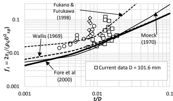
Fig. 4. comparison of measured friction factors with Wallis, Moeck, Fukano & Furukawa, and Fore et al. correlations.
