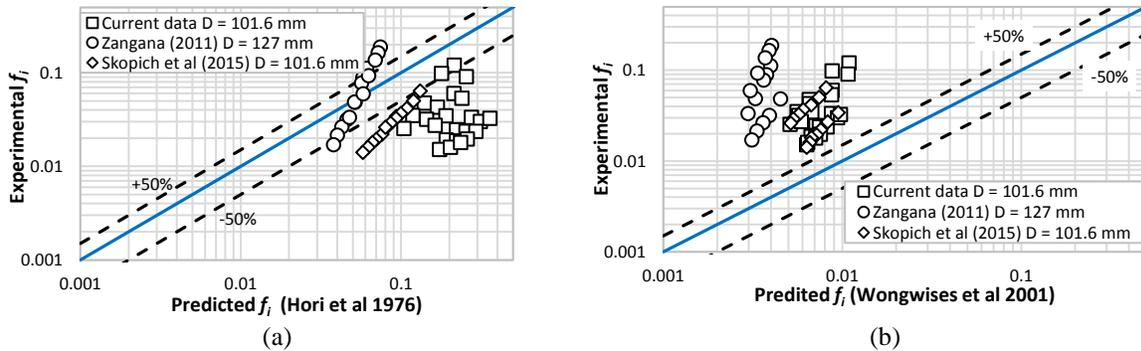
Fig. 5. Experimental vs friction factors predicted with Hori et al., Asali et al., Fukano et al., and Wongwises & Kongkiatwanitch correlations
