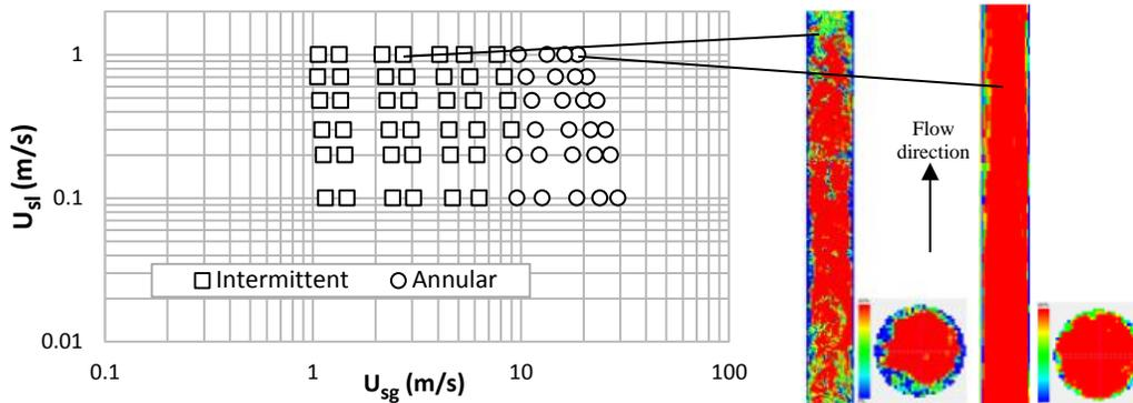
Fig. 2. Flow regime map by visual observation at the top position where the length to diameter ratio,  $L/D = 39$ , with reconstructed WMS images for  $U_{sl} = 1.0$  m/s;  $U_{sg} = 2.7$  and 18.6 m/s showing intermittent and annular flow regimes respectively. For the images, red colour signifies air while blue is water.
