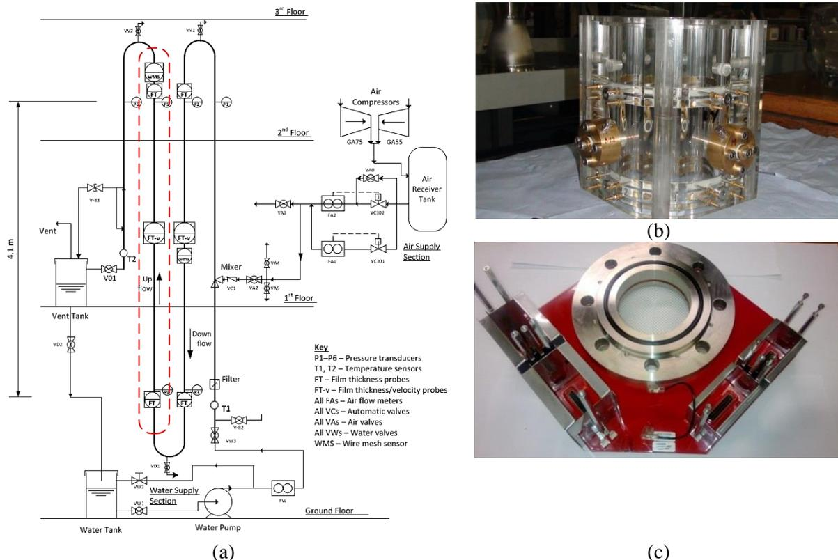
Fig. 1. (a) Cranfield University's Air-water two-phase serpent rig experimental facility (b) Conductance film thickness probe spool (c) Void fraction capacitance Wire Mesh Sensor (WMS)
