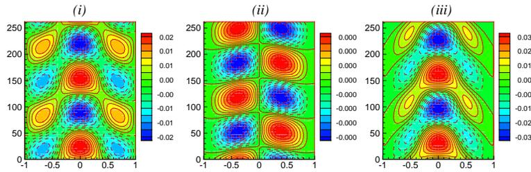
Fig. 5: Pattern of  $E^2$  component in the secondary flow at  $\delta = 0.5$ ; (i) disturbed  $u$ -velocity, (ii) disturbed  $v$ -velocity and (iii) disturbed temperature.
