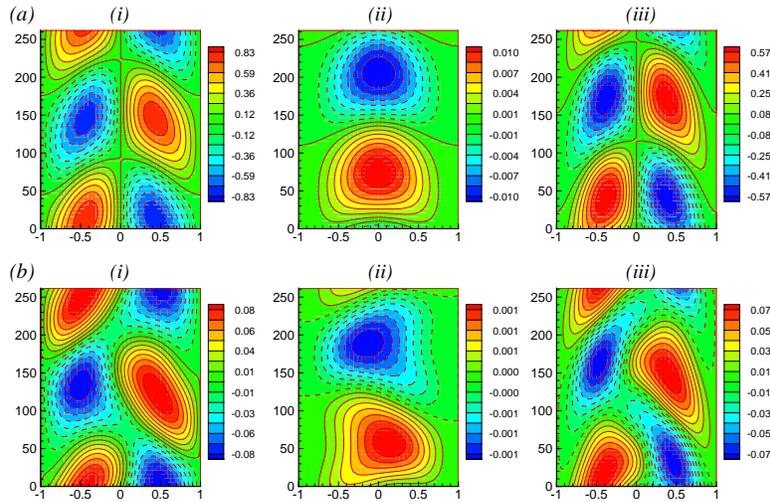
Fig. 4: Pattern of secondary flow by linear stability (a) and by nonlinear stability (b) at  $\delta = 0.5$ : (i) disturbed  $u$ -velocity, (ii) disturbed  $v$ -velocity and (iii) disturbed temperature.
