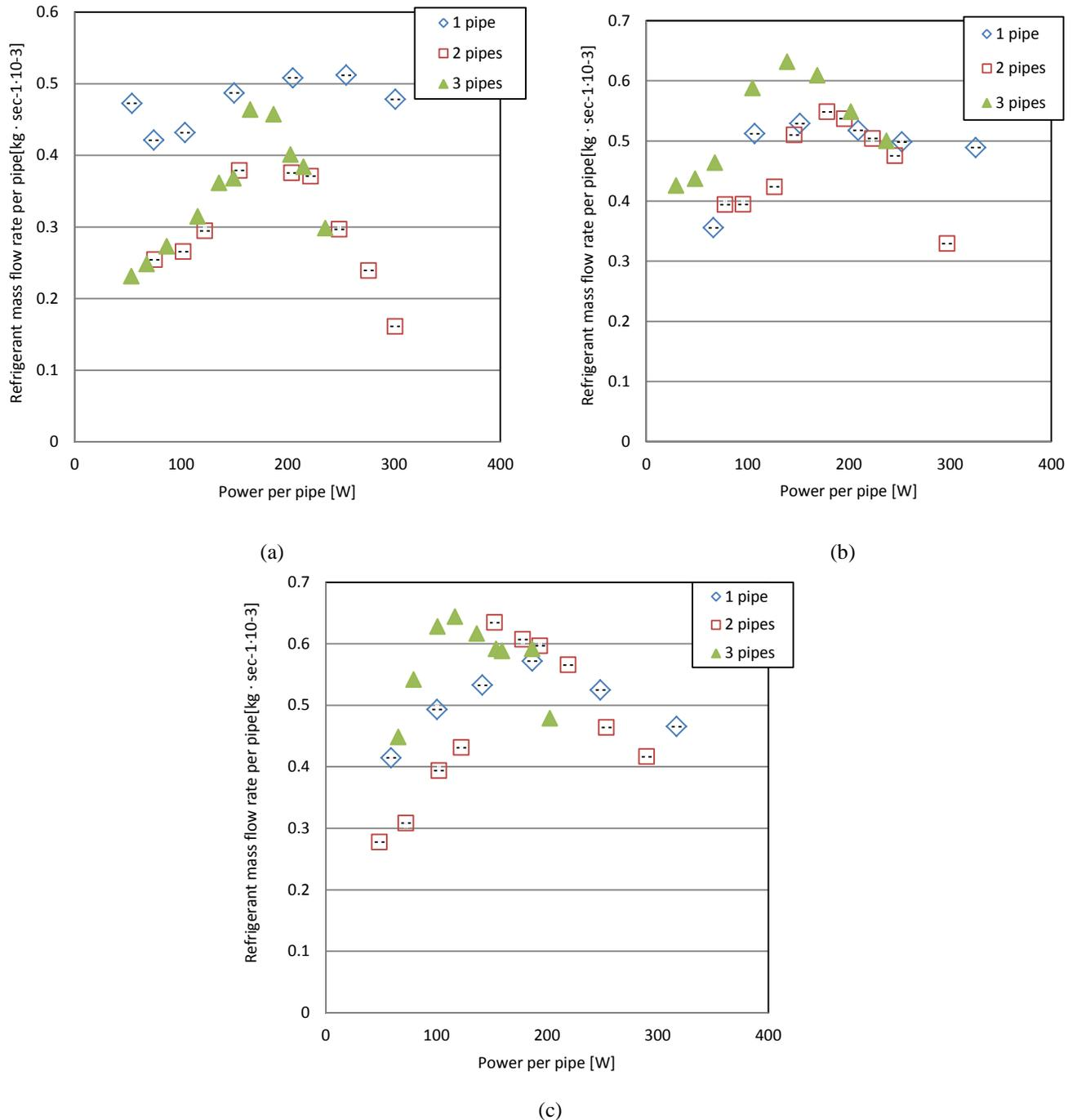
Fig. 5. Refrigerant mass flow rate vs. power input for one, two and three parallel lift tubes, motive head of 650 mm, 20% concentration (a), 30% concentration (b) and 40% concentration (c).
