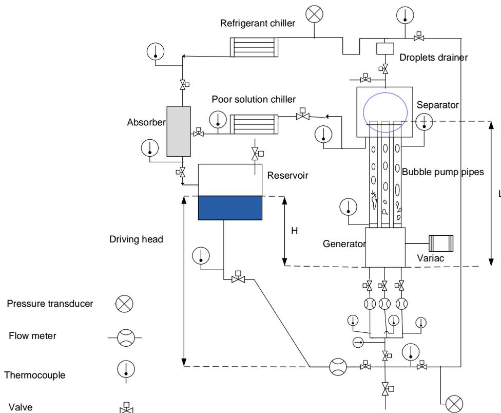
Fig. 2. Layout of the experimental system.
