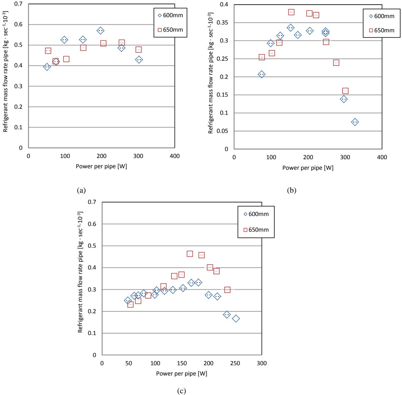
Fig. 4. Refrigerant mass flow rate vs. power input for 600 mm and 650 mm motive head, two parallel pipes, (a) 20% concentration, (b) 30% concentration, (c) 40% concentration.
