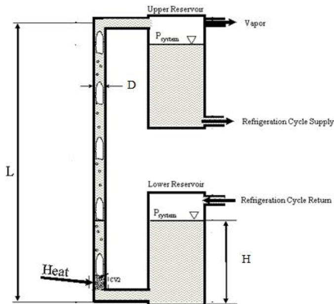
Fig. 1. Bubble pump schematic design.
