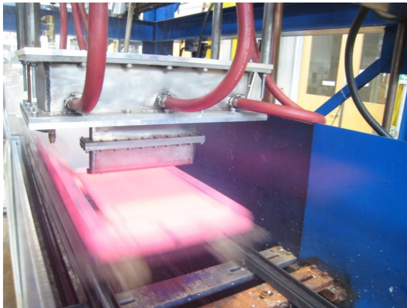
Fig. 3. Slant slit jet cooling system in operation
