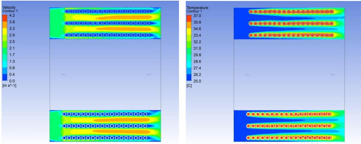
Fig. 2. Velocity and temperature fields for the pitch value of 6mm.
