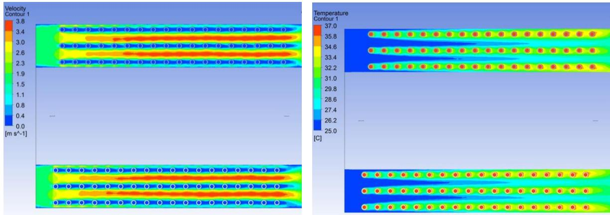
Fig. 5. Velocity and temperature fields for the pitch value of 12mm.
