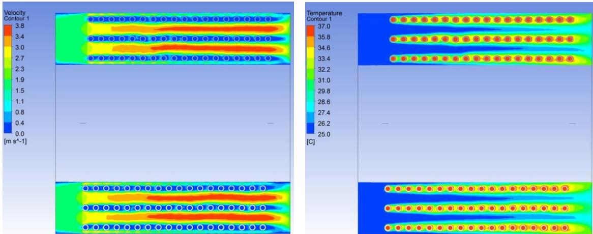
Fig. 3. Velocity and temperature fields for the pitch value of 8mm.
