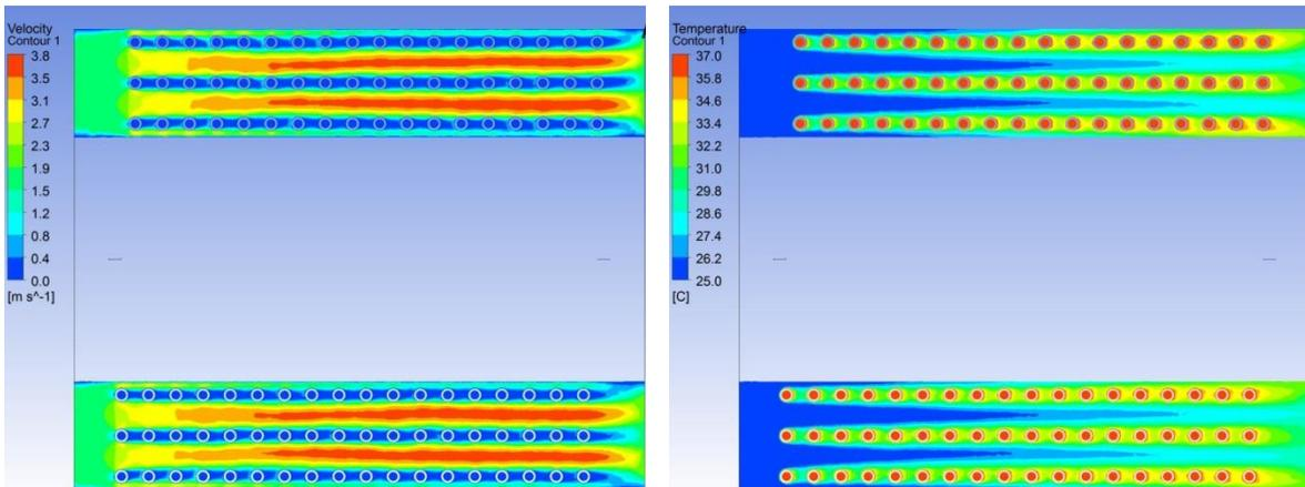
Fig. 4. Velocity and temperature fields for the pitch value of 10mm.
